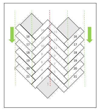
6. Now start on the other side and first of all install your supporting surface (with a perfect angle of 90°) in 45°. Now place half of the V shape and work in the other direction. Always press well on the long side to be sure that the 90 ° angle is maintained. Complete this line to the end of the room. You can do this left and right at the same time.
