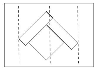
**3.** Place a support surface (with a perfect angle of 90°) at 45° so that the centre line runs through the centre of the top plank.
