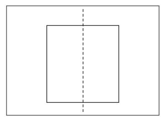
**1.** Measure precisely the width of the subfloor and determine the centre line in the middle.
