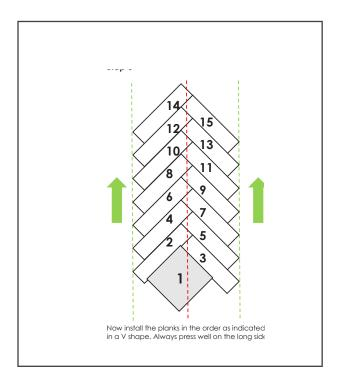
5. Now install the planks in the order as indicated above in a V shape. Always press well on the long side to ensure that the 90 ° angle is maintained. Complete this line to the end of the room.
